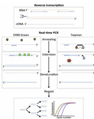
Source: Wikimedia Commons (n.d.) *Real-time PCR diagram showing SYBR Green and TaqMan chemistry*
