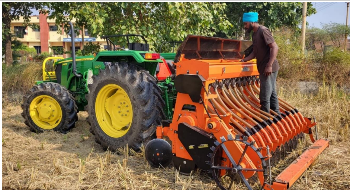
Fig.2: Sowing of Wheat seed by Super Seeder
